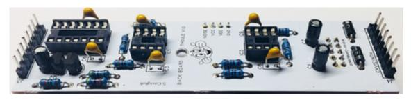
Place the IC chips with the right orientation
