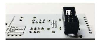
Solder 1 X connector. (This part will allow you to connect the Cavisynth Sample and Hold – OPTIONAL )
